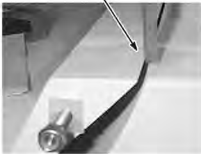
2mm to 4mm above End Bell surface.
