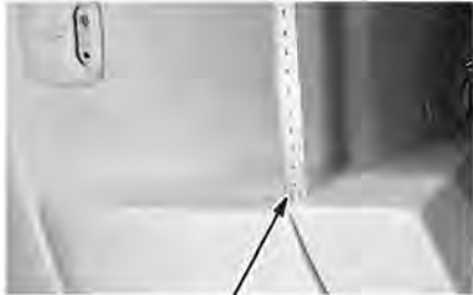
2mm to 4mm above End Bell surface.
