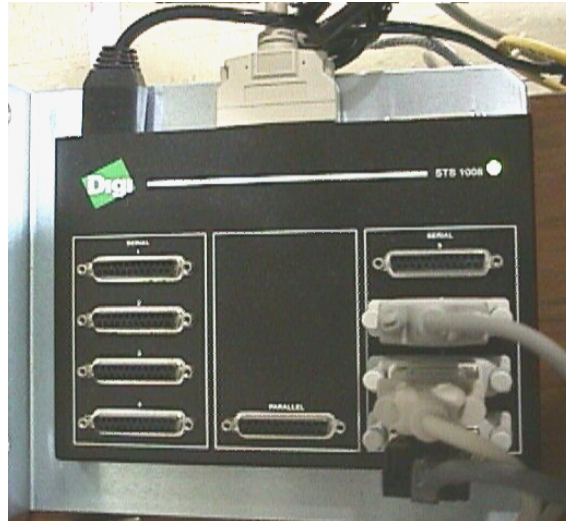
SCSI SERIAL EXPANSION BOX ILLUSTRATION 3-3
