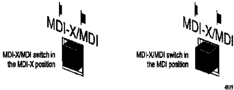
MDI/MDI-X SWITCH POSITIONS ILLUSTRATION 3-3
