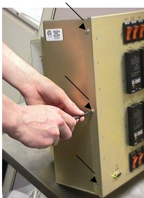
TCU SIDE SCREW LOCATIONS ILLUSTRATION 3-2
