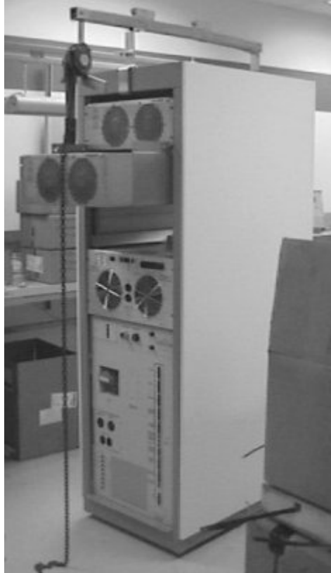
USING THE UNIVERSAL LIFT HOIST TO REMOVE THE RF AMP ILLUSTRATION A-9
