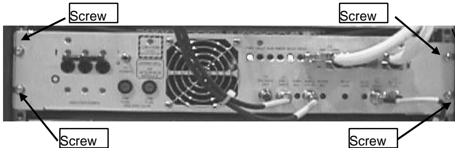
LOCATION OF SCREWS TO REMOVE RFI MODULE ILLUSTRATION 3-4
