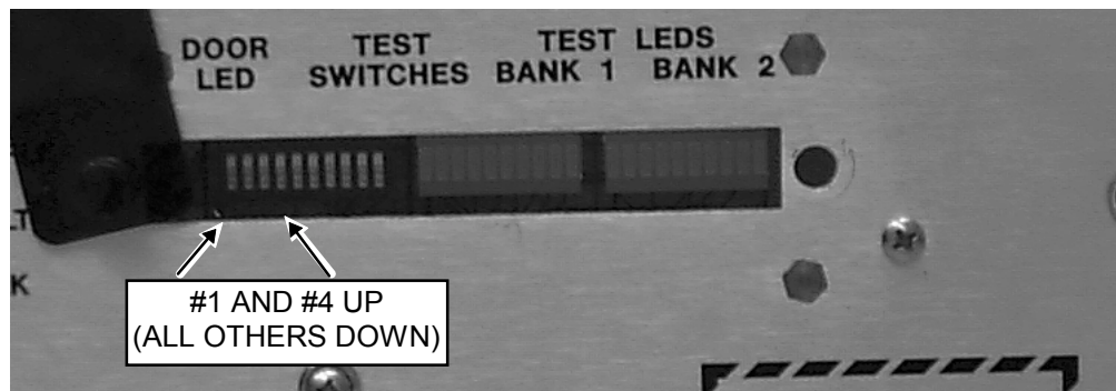
DIP SWITCH CONFIGURATION FOR PAC 8V ILLUSTRATION 5-3
