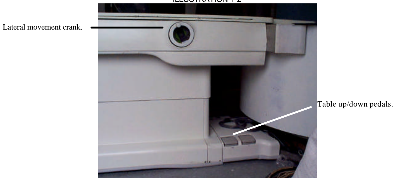
LATERAL POSITION ADJUSTMENT CRANK IS SHOWN AT TOP. VERTICAL POSITION CONTROL PEDALS
