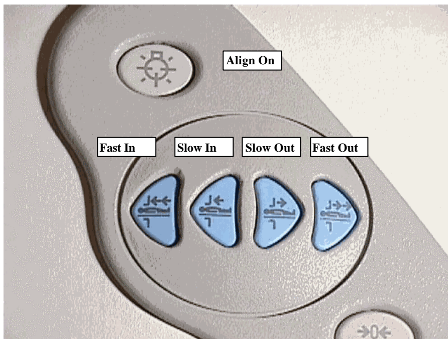
THE TOP LEFT BUTTON SHOWN IS THE ALIGN ON CONTROL THAT TURNS ON THE ALIGNMENT LIGHT.
