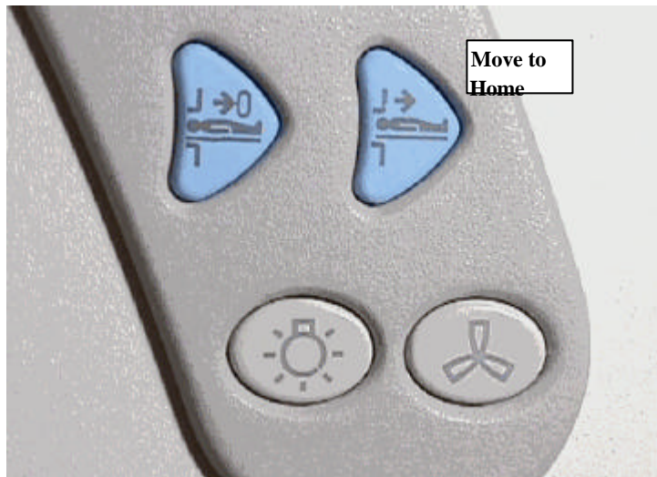
THE TOP RIGHT BUTTON SHOWN IS THE MOVE TO HOME CONTROL. ILLUSTRATION 1-2
