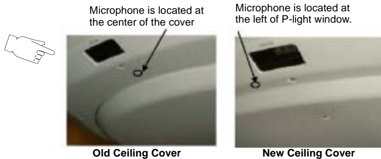
P-LIGHT COVER INSTALLATION ILLUSTRATION 8
