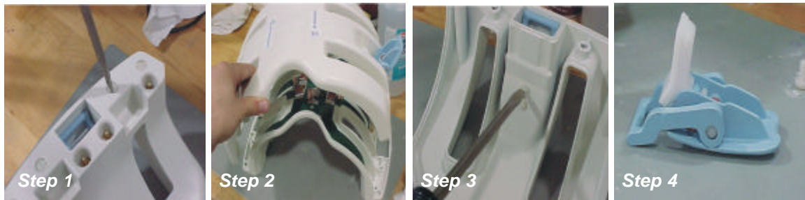
Figure 20: Replacing the latch mechanism.
