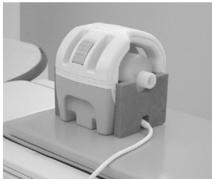
Figure 6: Positioning the knee phantom.
