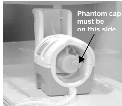
Figure 7: Positioning the foot phantom.
