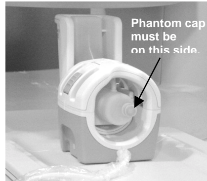
Figure 7: Positioning the foot phantom.
