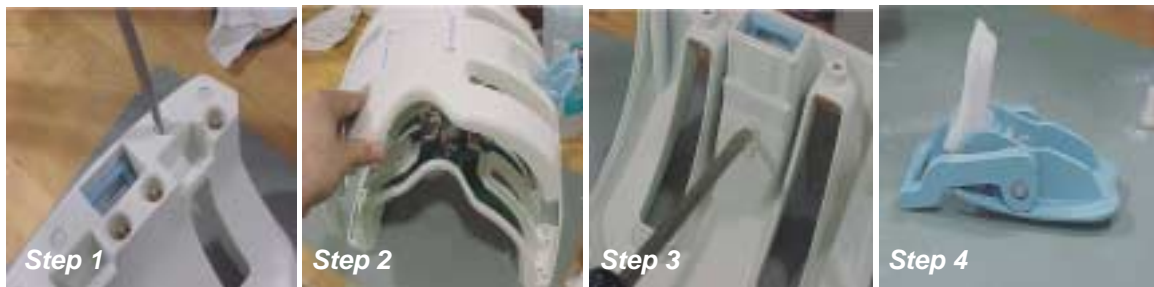
Figure 17: Replacing the latch mechanism.
