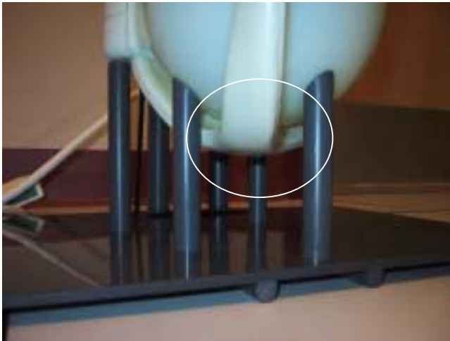
Figure 9: INCORRECT – Coil element IS NOT touching the phantom positioner pole.
