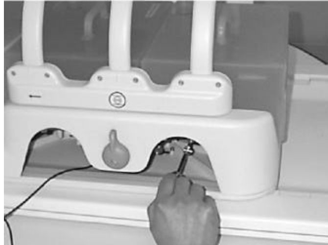
Figure 10: Adjusting the tuning capacitor.
