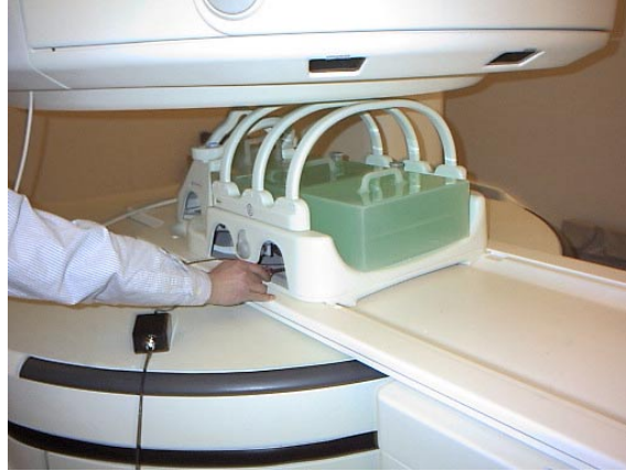
Figure 8: Phantom set on the coil in the system.
