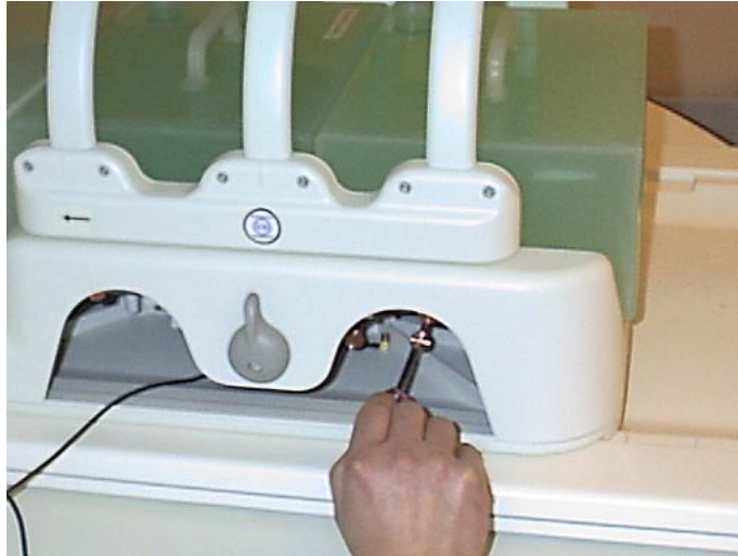
Figure 10: Adjusting the tuning capacitor.
