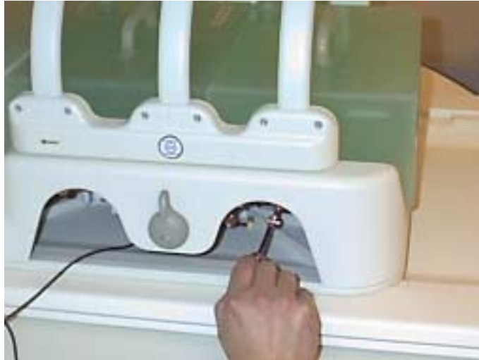
Figure 10: Adjusting the tuning capacitor.
