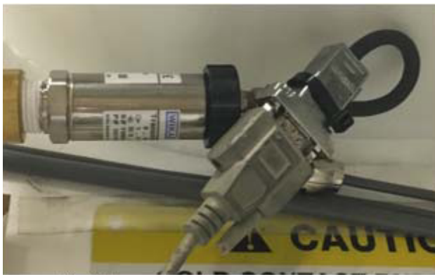
Figure 3-8 Attaching the pressure cable to the pressure transducer
