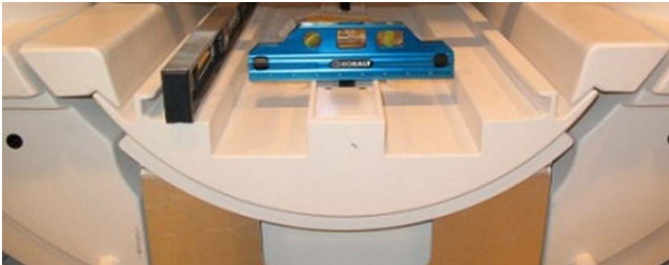
Figure 7-15 Magnet leveling, left-to-right
