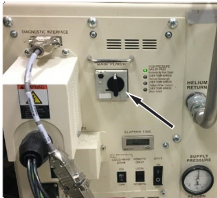
Figure 13 MAIN POWER switch
