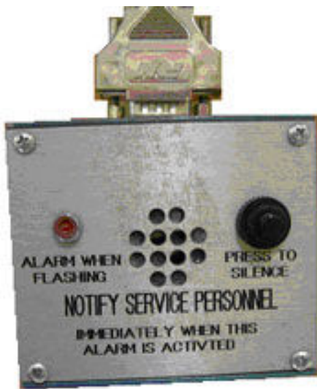
Figure 8 Remote alarm box
