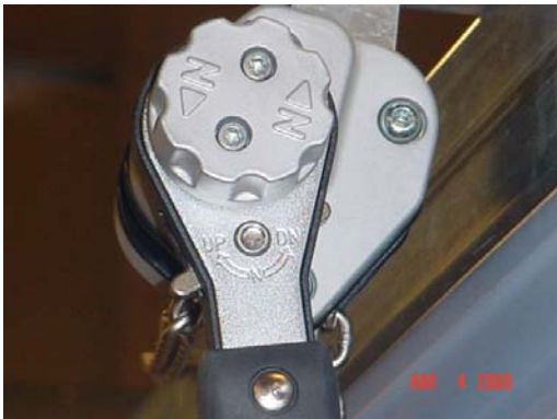
Photo 5 Hoist Handle in “UP” Position
