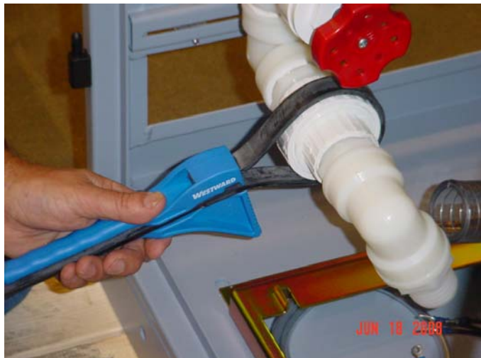
Photo 2 - Breaking the Suction Hose Connection to the Tank (Ebara Pump Only)
