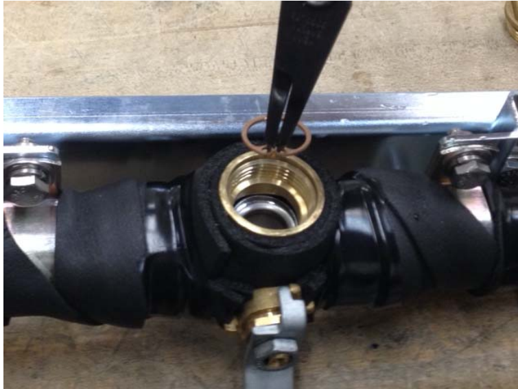
Illustration 5: Configuration #2 - Using Snap Ring Pliers to remove spring clip.
