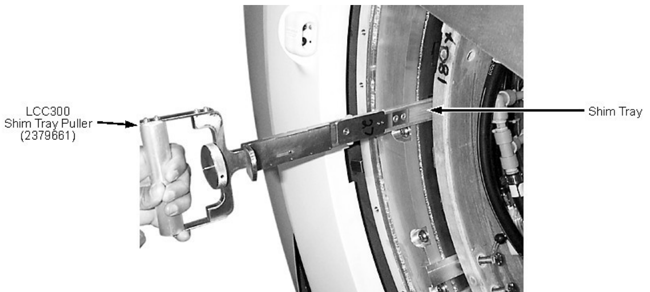
Illustration 3-138: Shim Tray Removal
