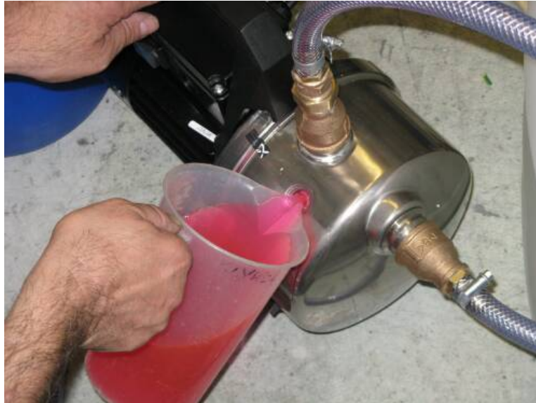
Figure 31 - Priming the filling pump
