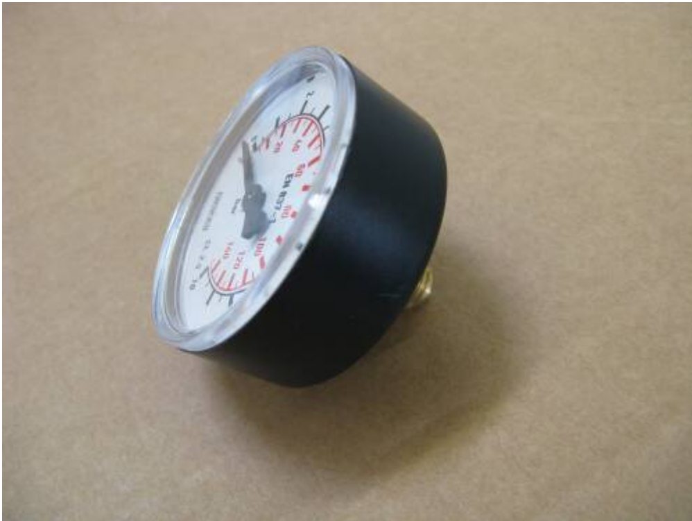
Figure 68 - The pressure gauge
