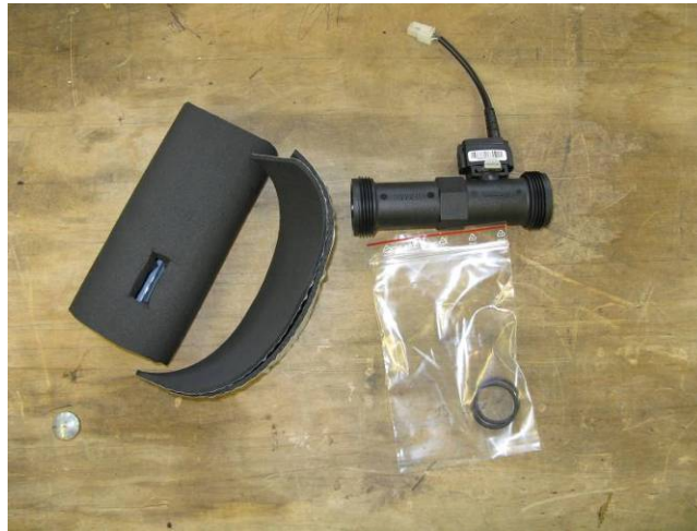
Figure 76 - LCC II primary flow and temperature sensor
