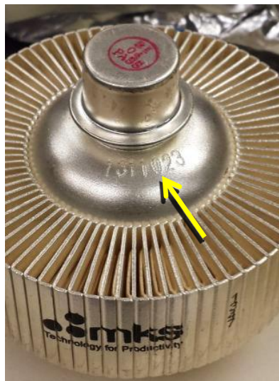
Figure 12 - MKS PA tube, with location of serial number
