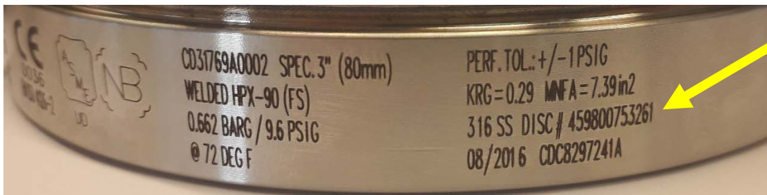
3-inch Metal Burst Disk 12NC location
