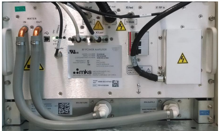
Water-cooled RF Amp
