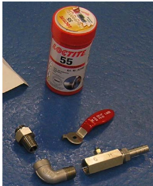
Figure 31 – The valve parts and Teflon tape
