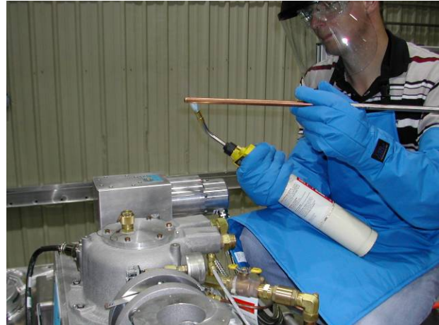
Figure 8.: Heating the 1/2" de-icing rod .
