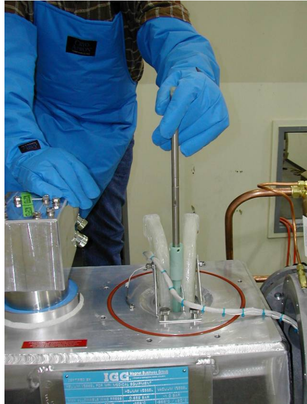
Figure 31. Using the alignment rod to direct the lead guides into place.
