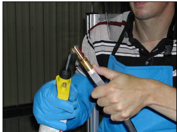
Figure 11. Heat the high-current lead to deice the lead guides. (Note the position of the thumb to monitor lead temperature.)
