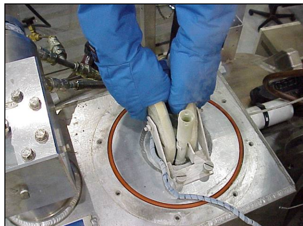
Figure 19. Lift the lead guides to see if they are frozen in place. DO NOT FORCE THEM.
