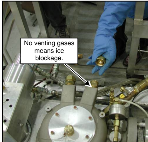
Figure 6. Check the negative high-current lead port for blockage.
