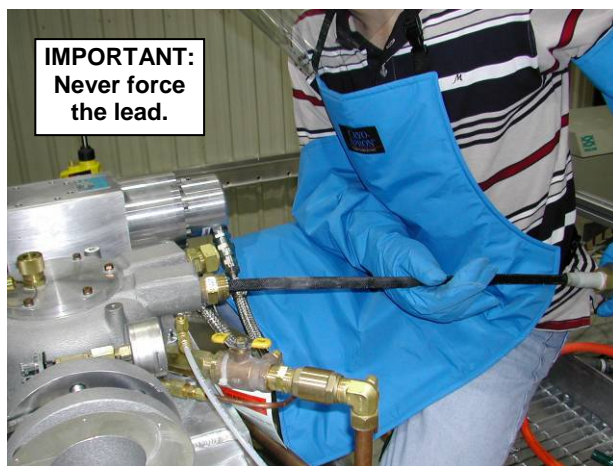
Figure 13. Carefully insert the high-current lead into the negative lead port.
