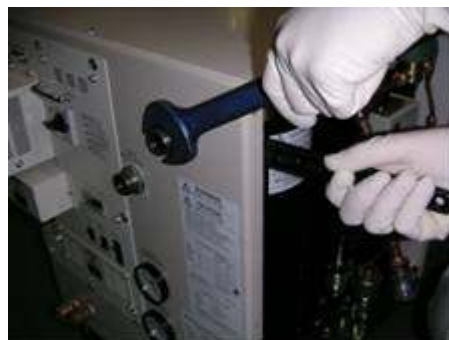
Tightening Torque: 23 Nm
