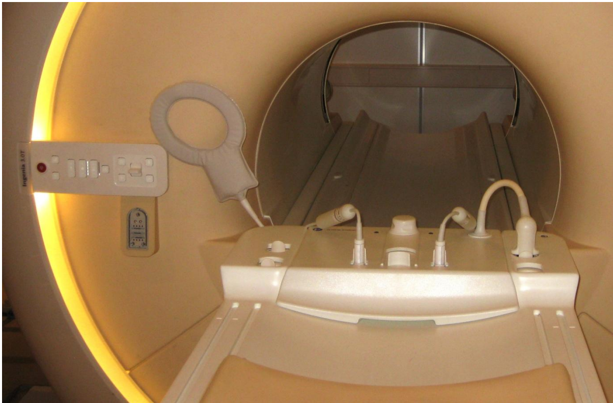
The flex-M coils connected to the dStream interface. During 'real life' spike searching the covers are removed
