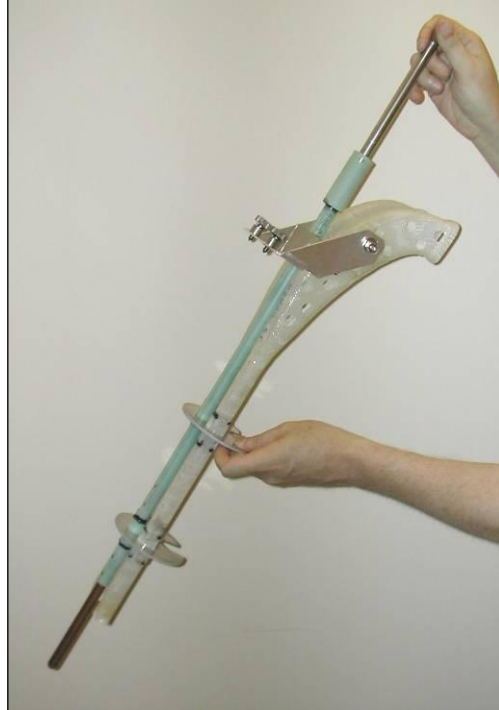
Figure 8-8 - Use an alignment rod to help direct the lead guides into place (OPEN-X / Rex style shown).
