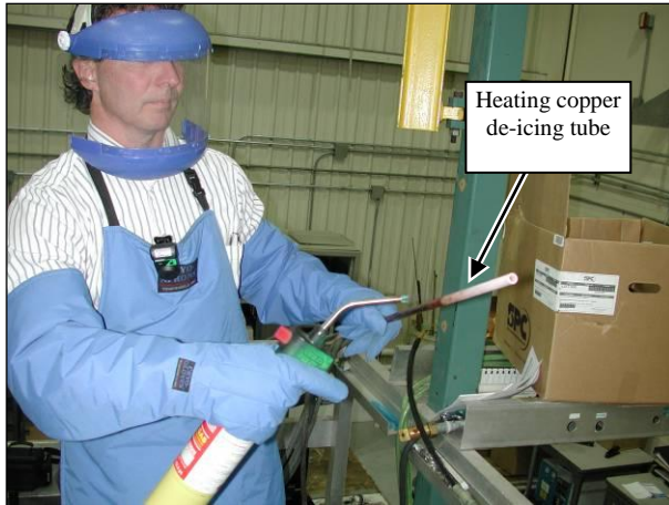
Figure 5-2 - Heating the 1/2" copper de-icing rod to create a vent.
