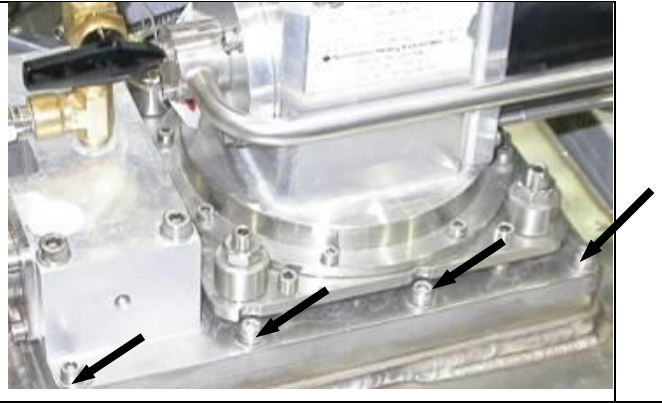
Figure 6-5 – Rectangular-flange with ten M6 (5mm socket head) hold-down screws (six are not shown)
