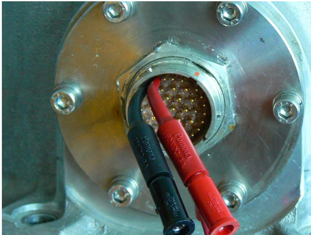
Figure 5 – Test adaptors connected to read thermistors
