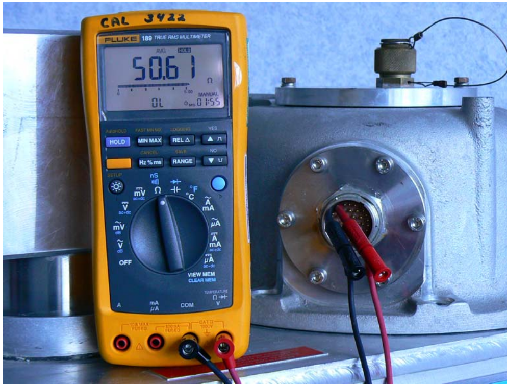
Figure 4 – DMM Set-up to read thermistors
