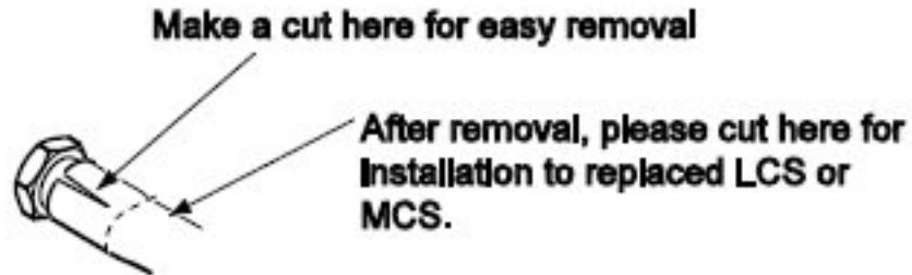
Illustration 2-40: Removal of hose
