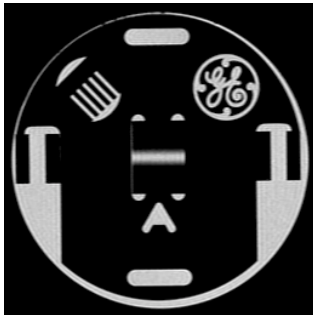
ILLUSTRATION L1 IMPROPERLY CENTERED DQA-III INTERNAL STRUCTURES
