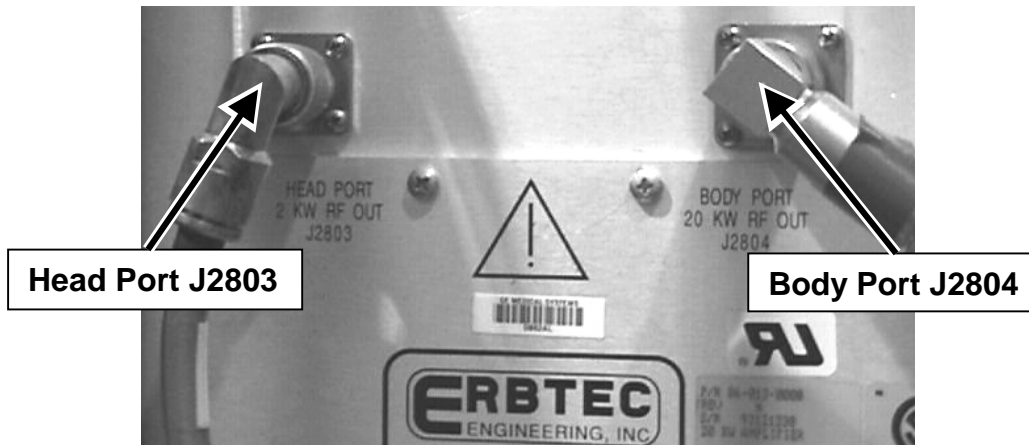
ERBTEC RF AMPLIFIER HEAD AND BODY PORTS ILLUSTRATION 3-2
