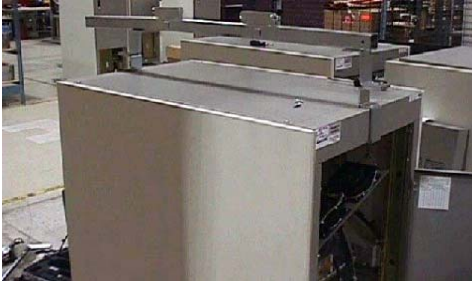
HOIST INSTALLED ON TAC CABINET ILLUSTRATION 9-6
