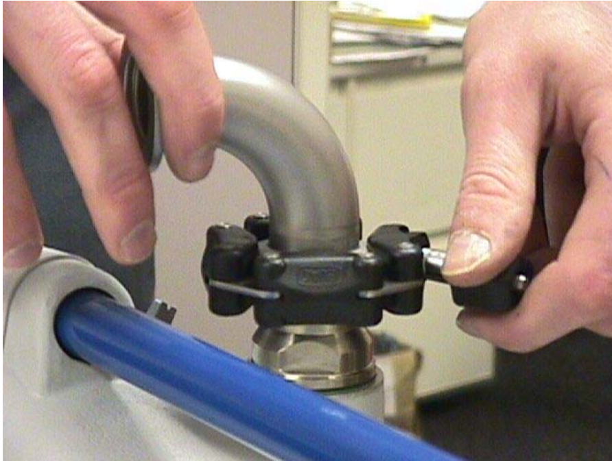
VACUUM CLAMP AND ELBOW ILLUSTRATION 9-20
