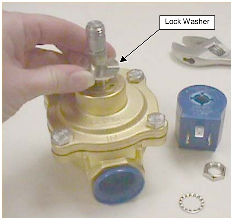
REMOVING LOCK WASHER ILLUSTRATION 9-27
