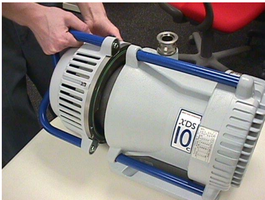
REMOVING THE REAR OF THE VACUUM PUMP ILLUSTRATION 9-13
