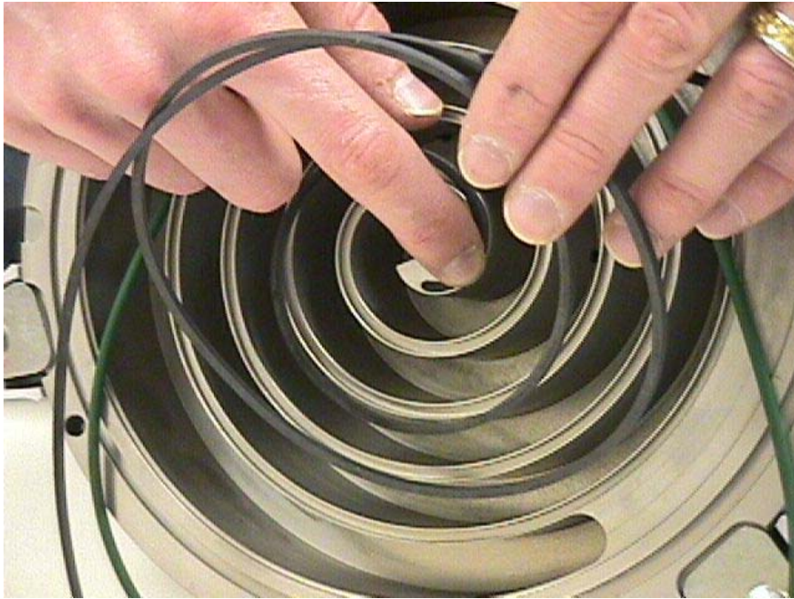
TIP SEAL INSTALLATION ILLUSTRATION 9-16
