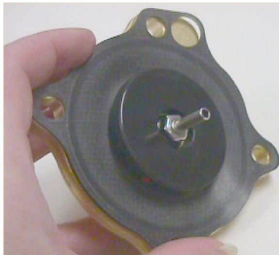
NEW RUBBER DIAPHRAGM ON TOP-PLATE ILLUSTRATION 9-38
