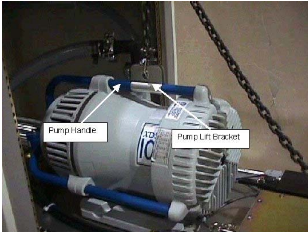
VACUUM PUMP LIFT BRACKET ILLUSTRATION 9-11
