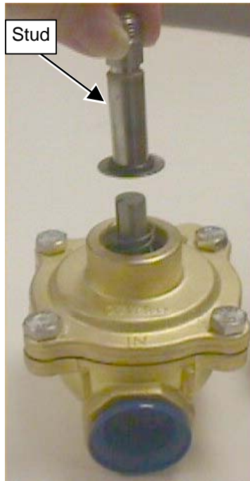
REMOVING STUD ILLUSTRATION 9-29
