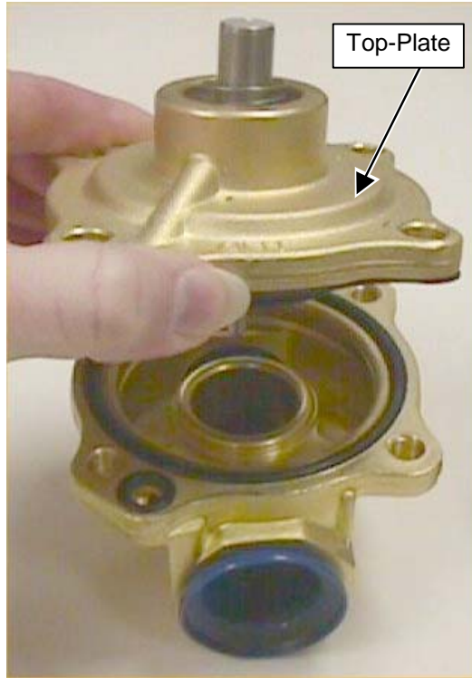
REMOVING TOP-PLATE OF SOLENOID VALVE ILLUSTRATION 9-31
