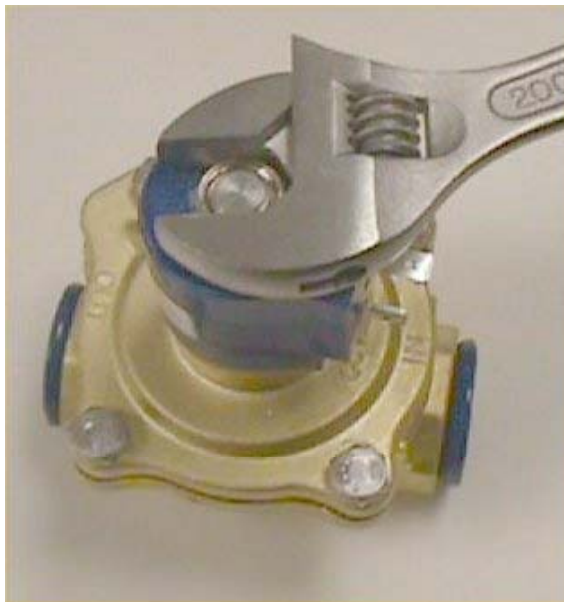
REMOVING TOP NUT FROM SOLENOID VALVE ILLUSTRATION 9-25
