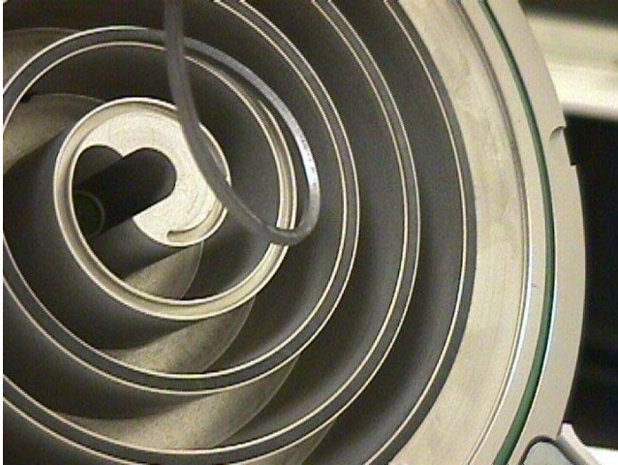
TIP SEAL REMOVAL ILLUSTRATION 9-15
