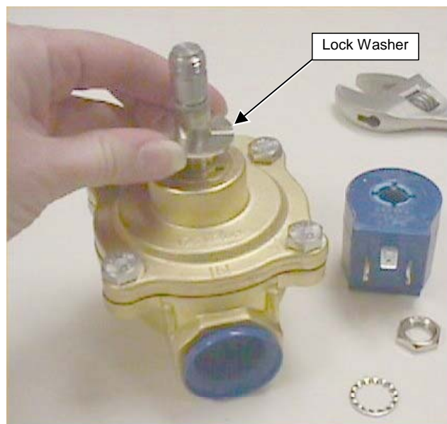
REPLACING LOCKING WASHER ILLUSTRATION 9-42
