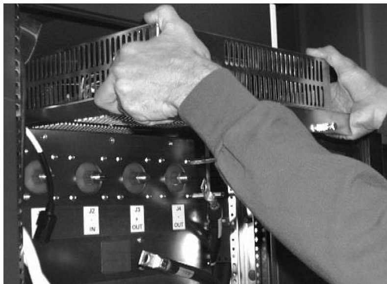
REMOVING THE FAN MODULE ILLUSTRATION L4581B
