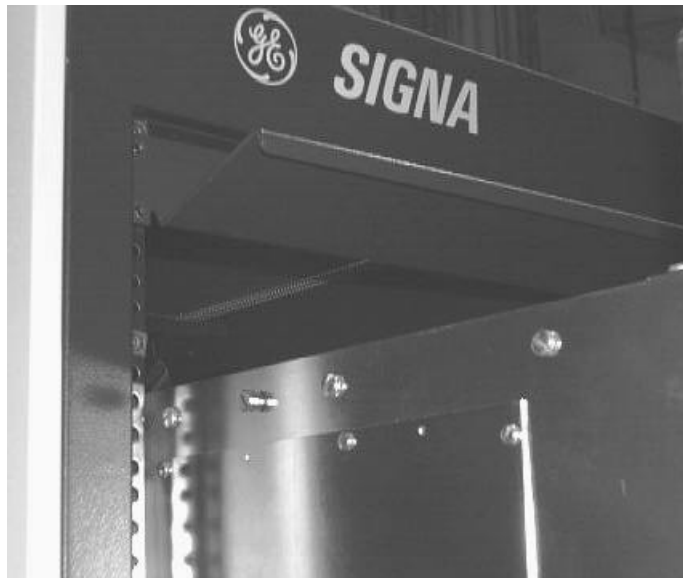
SHOULDER SCREW FOR ATTACHING HOIST LIFT PLATE ILLUSTRATION L4586A
