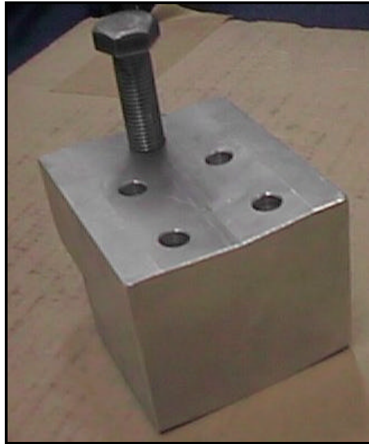
BOLT PLACED IN COIL INTERFACE BRACKET
