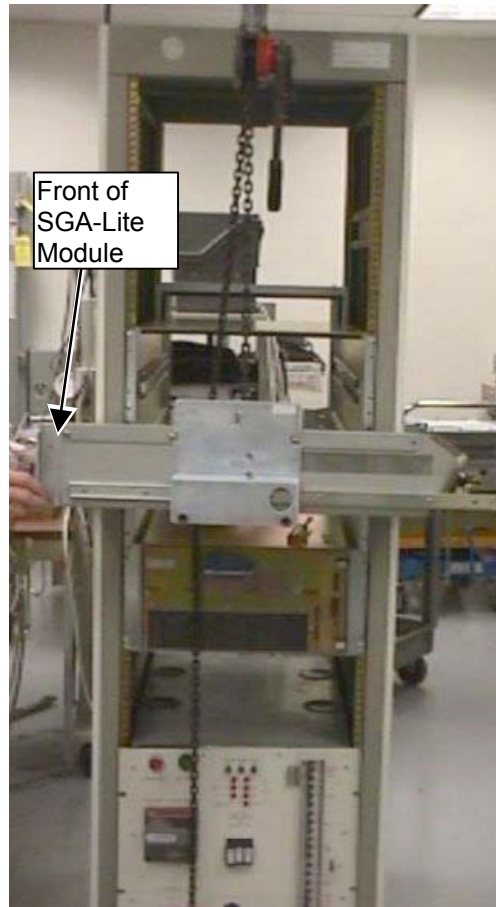
TURNING MODULE TO THE SIDE TO LOWER FROM CABINET ILLUSTRATION 1-17
