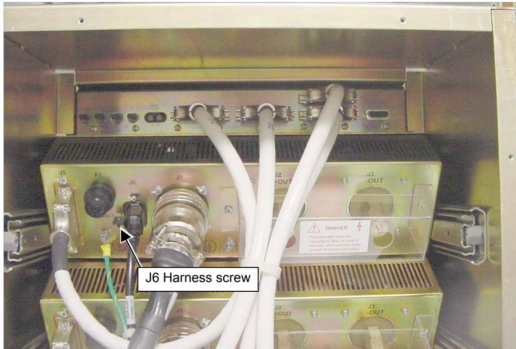
SECURING AC POWER CORD ILLUSTRATION 1-19
